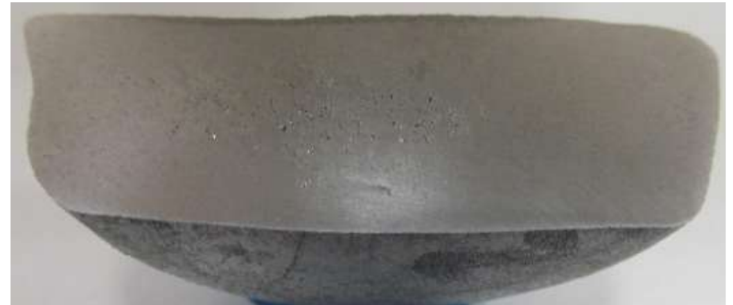
Degassed: RPT Density 2.66, AISCAN (0.128 ml/100g)
