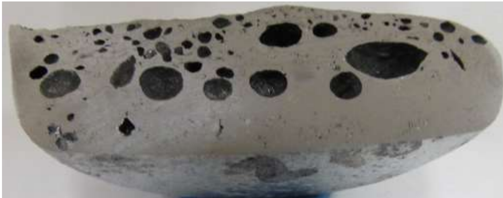
Untreated: RPT Density 2.18, AISCAN (0.365 ml/100g)
