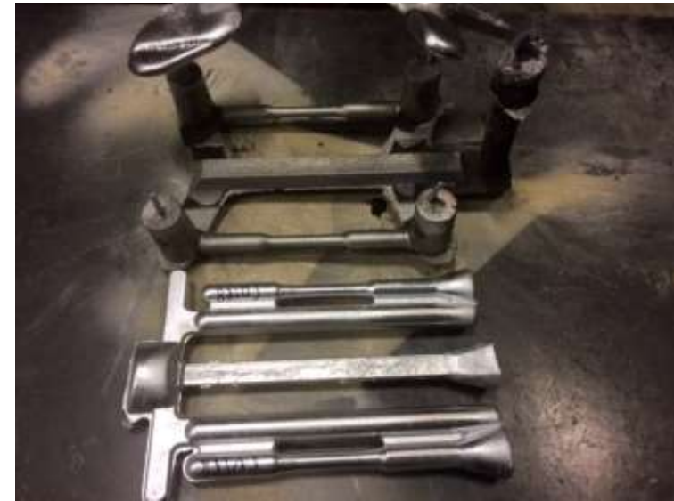
As cast test bars, ASTM B26 sand mold above and B108 permanent mold below
