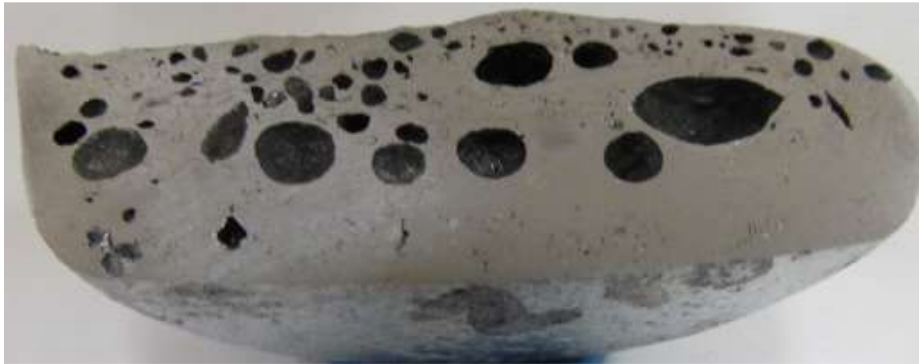
Untreated: RPT Density 2.18, AISCAN (0.365 ml/100g)
