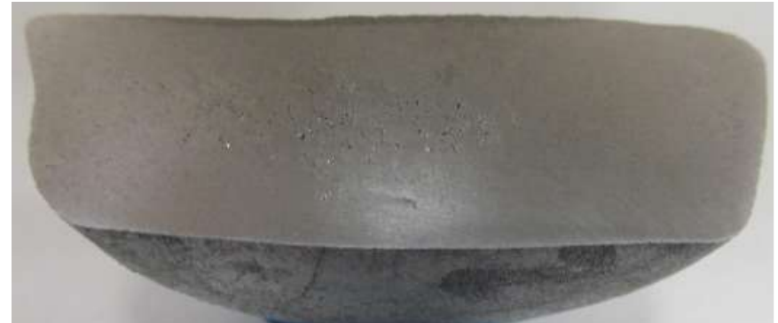
Degassed: RPT Density 2.66, AISCAN (0.128 ml/100g)
